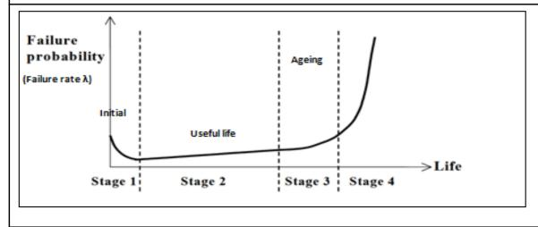
Model for the probability of failure of a population of equipment: the "bathtub curve" shows the typical four stages of the progressive ageing
