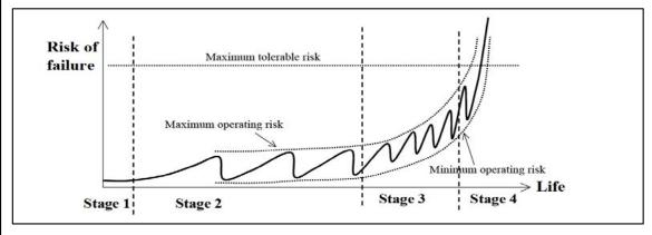
Effect of **periodic maintenance** on the risk of failure, varying **between tolerable risk and operating risk**
