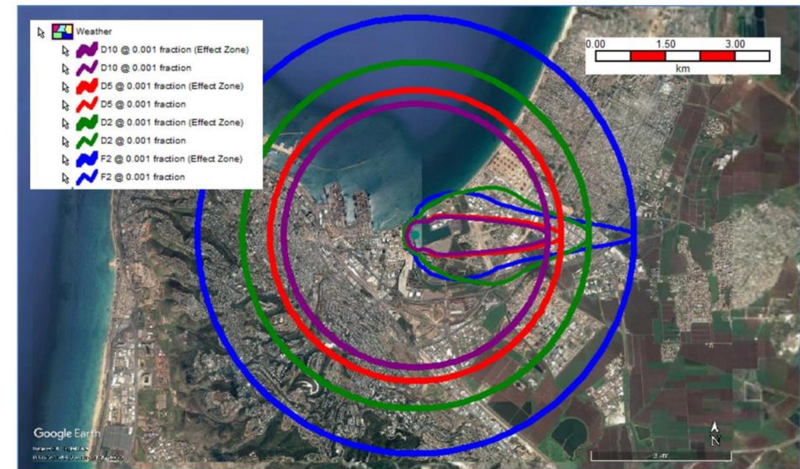
Figure 5-13 0.1% Lethality Footprint and Effect Zone for Liquid Carrier (2500 te) Catastrophic Release (to the Sea)
