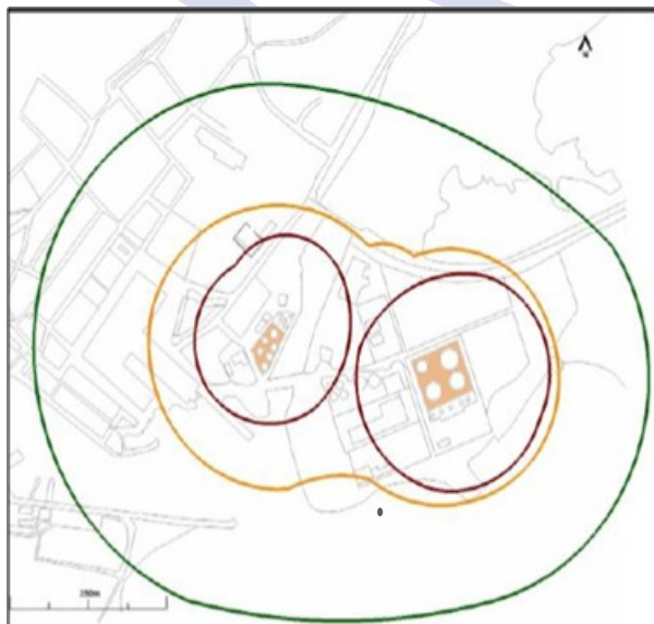
Figure 3 Example of a Public Information Zone applying the approach of the Irish Health and Safety Authority.
