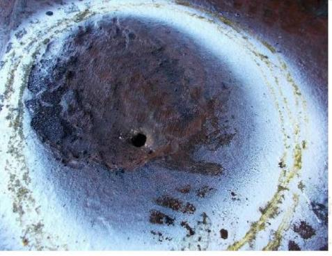
Three through-holes in the central plates localized corrosion
