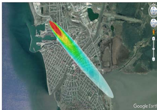
Figure 2 Visualization in ADAM of spatial dispersion of a toxic plume on a local map
