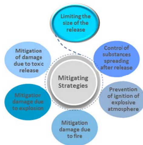
Figure 1. Emergency isolation systems can limit the size of the release and mitigate incident effects.
