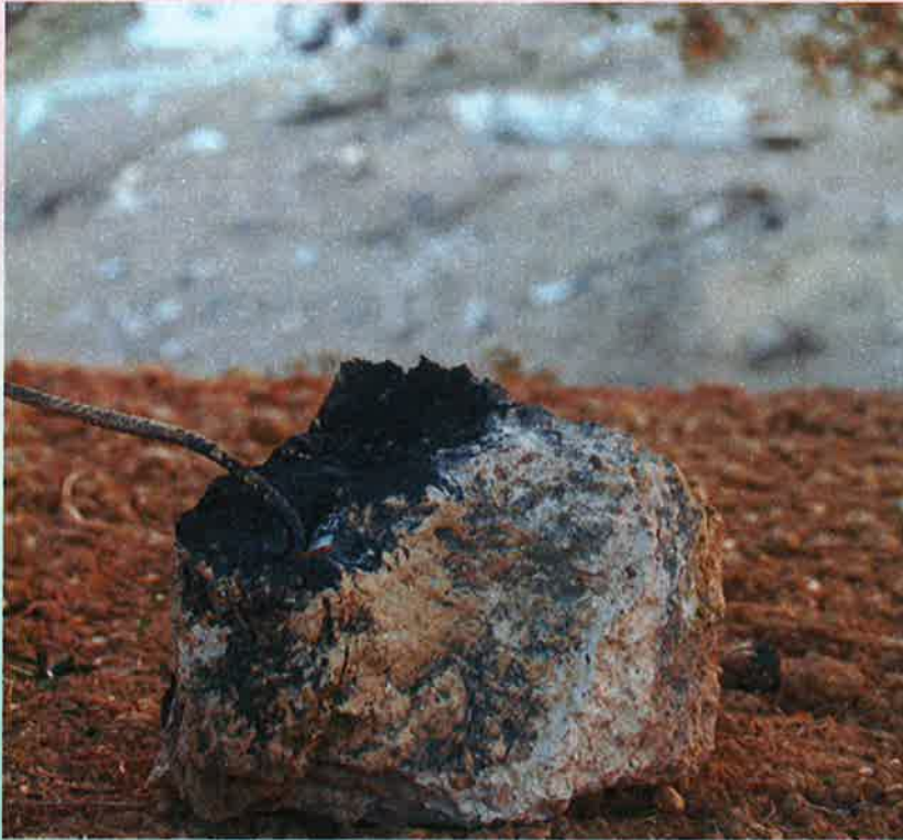
Piece of concrete found more than 900 m away from the plant
