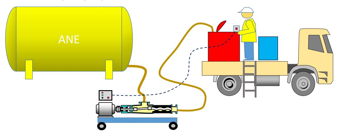
MANUAL MONITORING OF THE LEVEL IN THE ANE TANK WHILE FILLING THE TANK ່ບດດ
