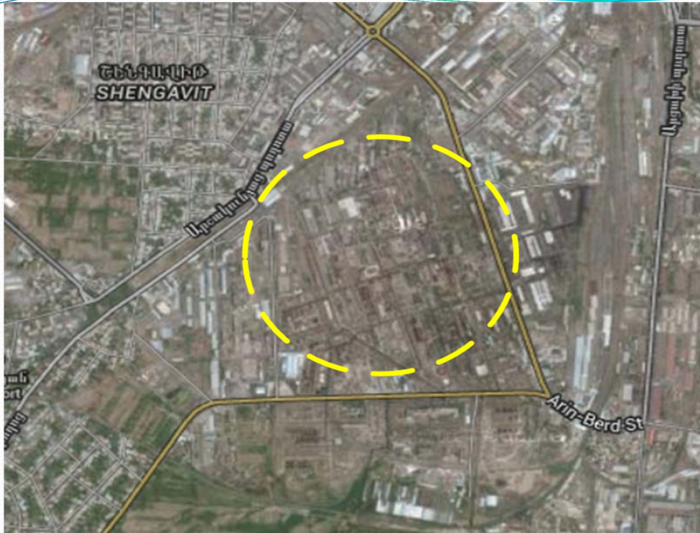
Hazard Map 1Narit, YerevanThe 1 km radius is plotted indicating the Exposure Distance for Human Direct - Health regarding Ammonia.
