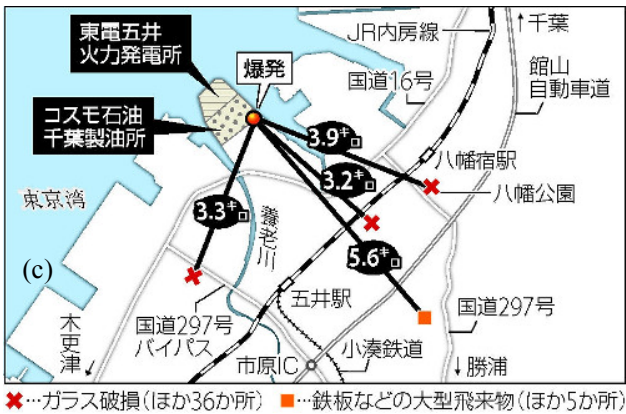
Fig. 7 (a) Collapsed Tank resulting from the damaged bracing (b) A photo just before the explosion (c) Range of flying debris projectiles
