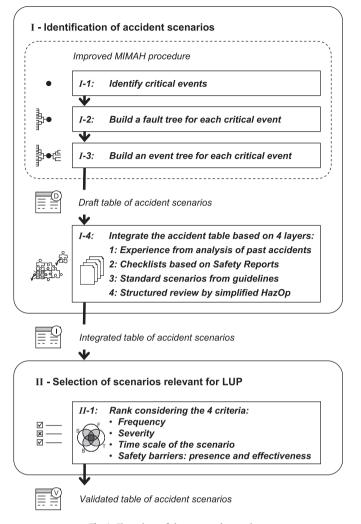
Fig. 1. Flow chart of the proposed procedure.
