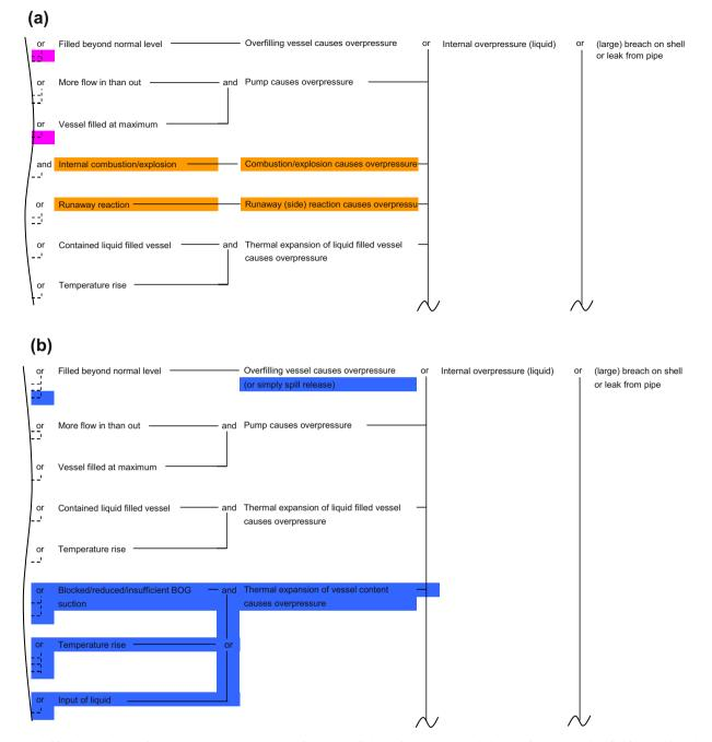
Fig. 3. Example of fault tree adaptation for an LNG storage tank: a) section of the generic fault tree from MIMAH; shaded areas refer to causes identified for possible exclusion on a preliminary basis; b) section of the validated fault tree; shaded areas refer to causes modified during the review and validation process.
