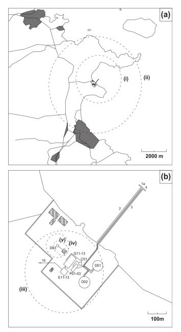
**Fig. 7.** Case-study 2: fictitious plant location (panel a) and layout (panel b). Dashed lines mark worst case damage contours discussed in the text for selected units: (i) LNG unloading arm (stream 1a); (ii) LNG storage tank (D01); (iii) vaporizer (E12); (iv) diesel tank (D03); (v) diesel pipework (stream 17).
